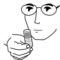
**Post-analysis sterilization** is performed by exerting gentle pressure on the cap and allows the safe disposal of the vial.
